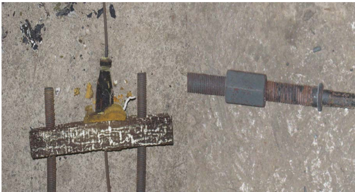
Figure 17 Fixings on removal from the furnace
