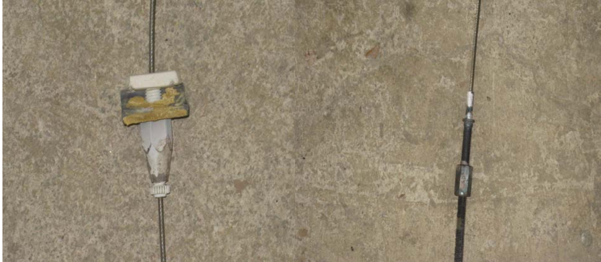
Figure 6 Fixings on removal from the furnace
