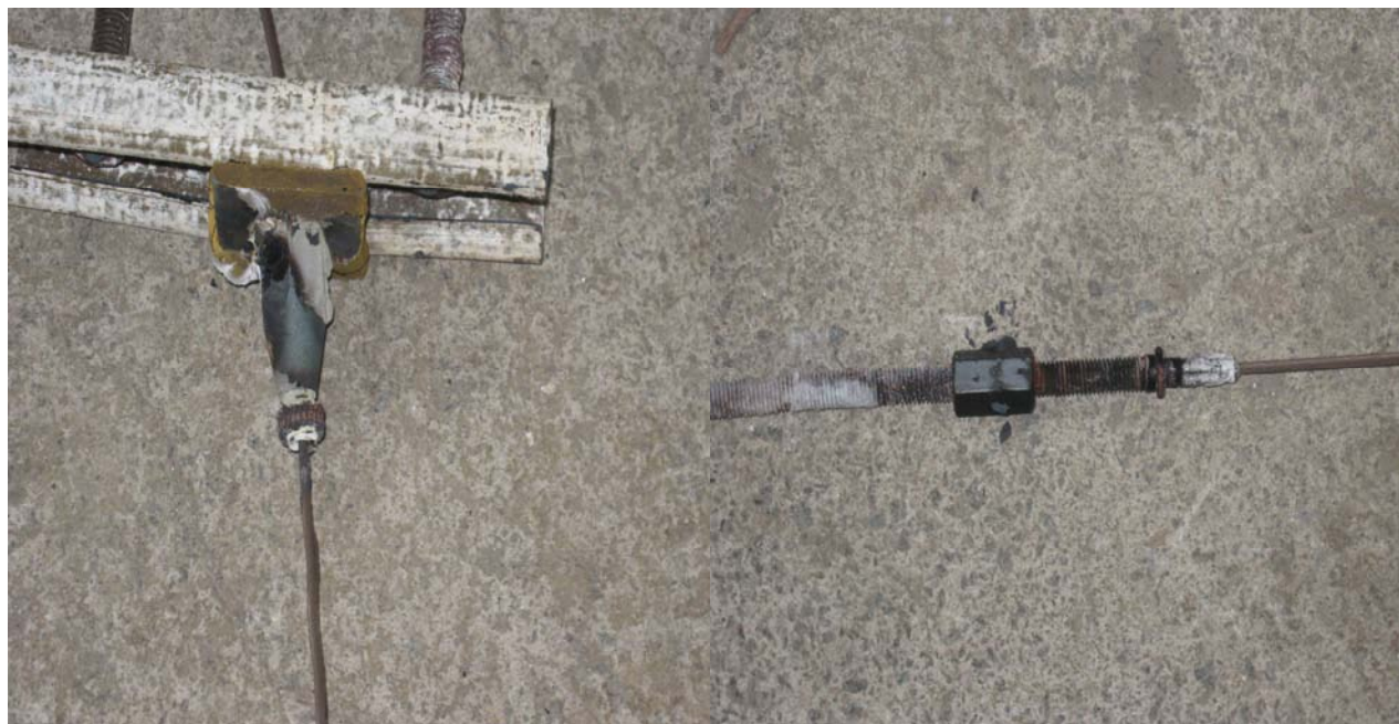
Figure 13 Fixings on removal from the furnace
