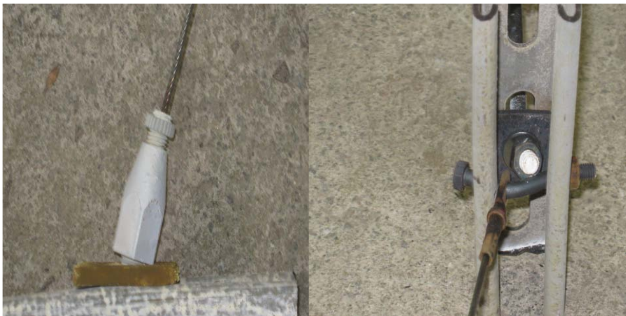
Figure 11 Fixings on removal from the furnace
