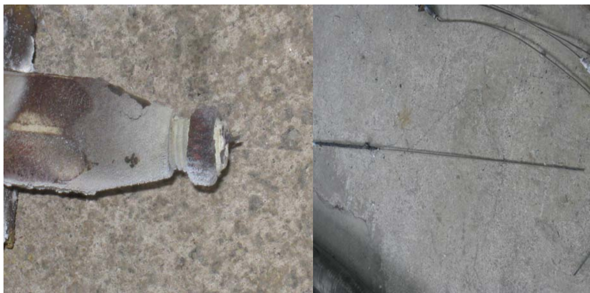
Figure 15 Fixings on removal from furnace
