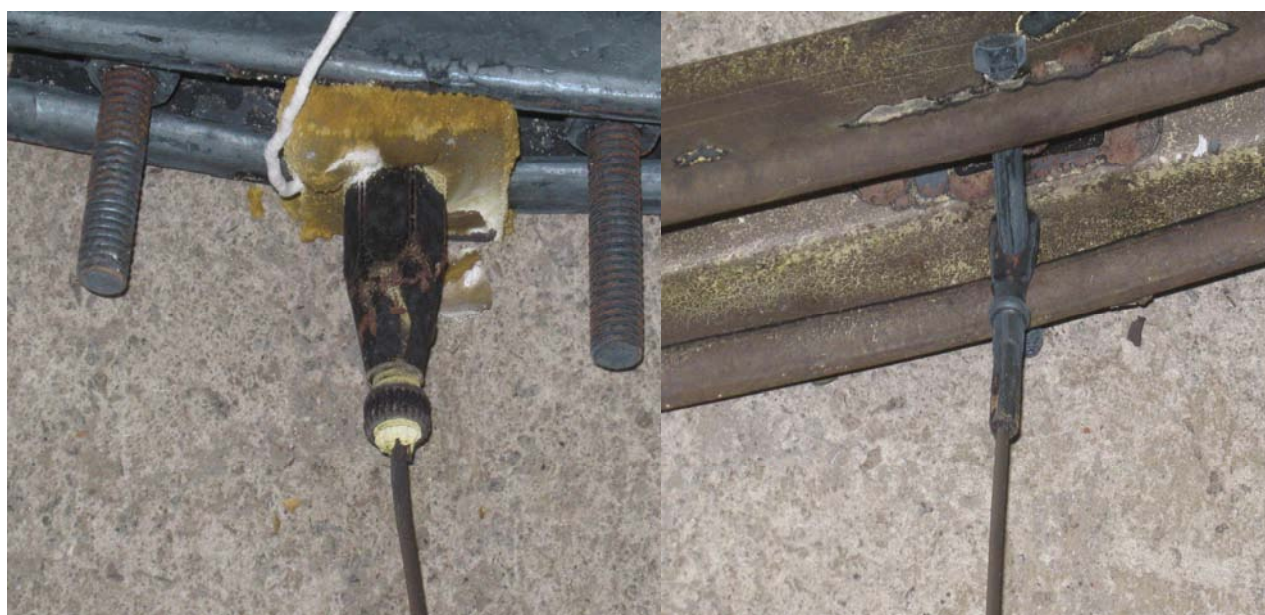
Figure 23 Fixings on removal from the furnace
